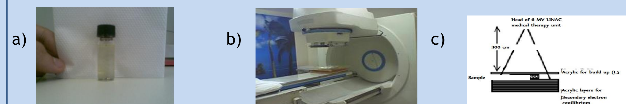
Fig.2. Irradiation Conditions: a) dosimetric solutions in 4 mL vial b) 6 MV medical linear accelerator c) Irradiation dimensions
