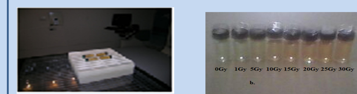
Fig.3. Visual color changes of Cy7-PF6 solution in chloroform irradiated at (a) 30 Gy and (b) color
