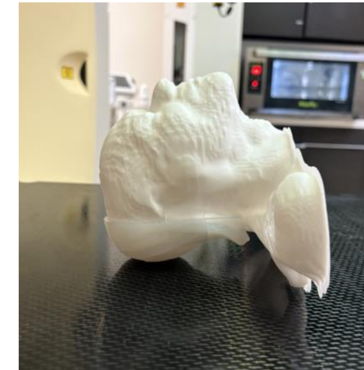
Figure 4. 3D printed Head and Neck Phantom with silicone bolus at CT SIM
