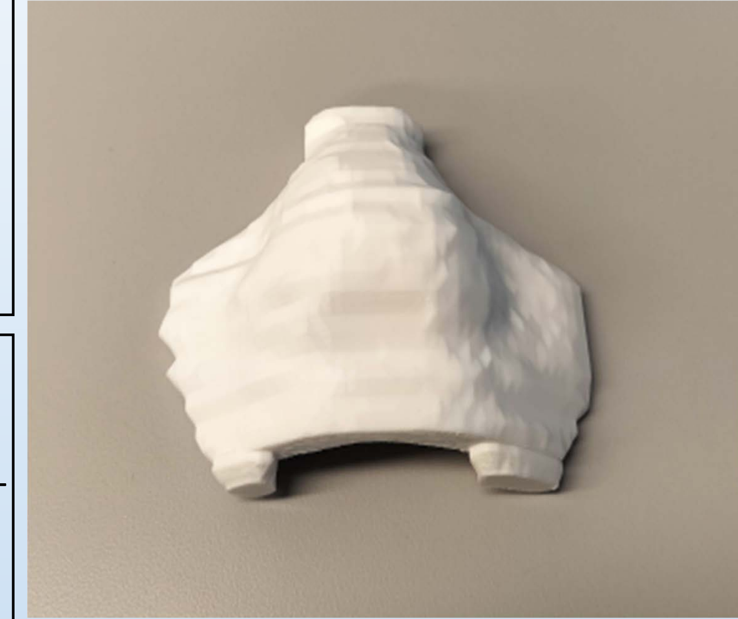
Figure 3. Excess materials were removed from printed bolus. Sharp edges were smoothed out and rounded off.
