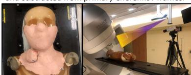
Fig. 1. Phantom and camera setup (top). Image acquisition process via time gating to linear accelerator pulses (bottom).
