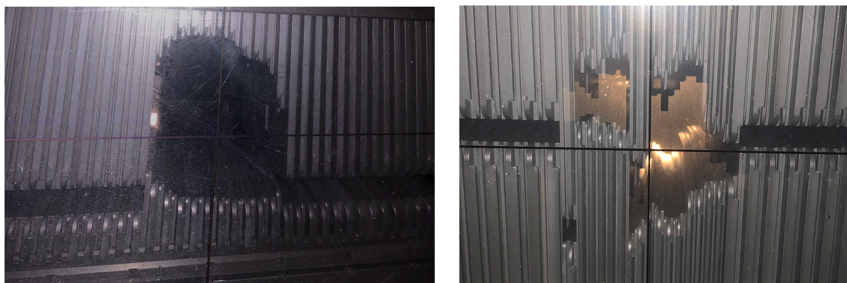
Figure 3. MLCs of Edge with 0.25 and 0.5cm leaves (Left) and TrueBeam with 0.5 and 1.0cm leaves (Right).
